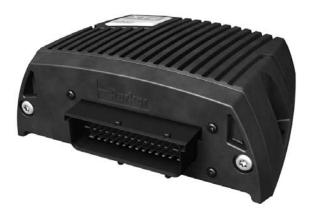
Weight Operating temperature Protection Voltage supply Current consumption (idle) 0.7 Kg -40 to +70 °C outdoor use 9 - 34 VDC 105 mA (28 VDC) 90 mA (14 VDC) Parker ICP (IQAN CAN Protocol)
