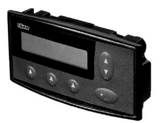
Weight Rated power supply Min/max power Operating temperature (reduced display update) Protection Current consumption 0,2 kg 12-24 Vdc 9/32 Vdc -30°C to +70°C -30°C to -10°C outdoor use max 100 mA (28 Vdc), max 180 mA (14 Vdc) Parker ICP (IQAN CAN Protocol)
